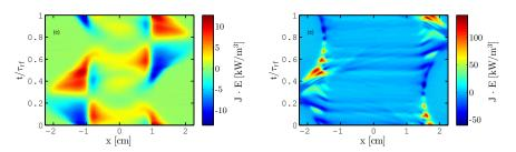
■ The spatio-temporal electron heating at 10 mTorr with a gap separation of 4.5 cm driven by a 222 V voltage source at 13.56 MHz (left) and 27.12 MHz (right)
