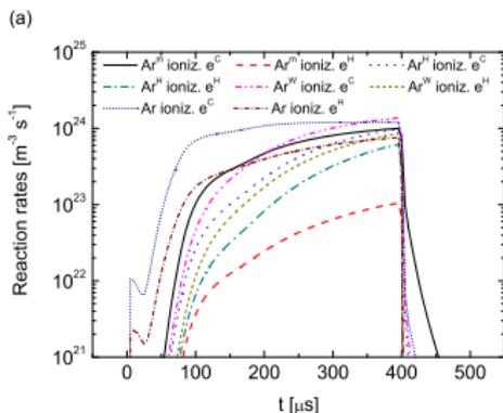
The temporal variations of the reaction rates for electron impact ionization of the argon atoms (ground state plus metastable) in poisoned mode.
