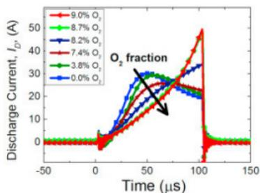
The current waveforms for an Ar/O<sub>2</sub> discharge with a V target where the oxygen flow rate is varied
