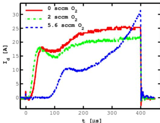
The current waveforms for an Ar/O<sub>2</sub> discharge with a Ti target where the oxygen flow rate is varied – 600 V, 50 Hz and 0.6 Pa
