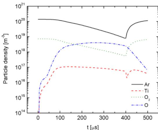
The temporal evolution of the neutral species with 5 % oxygen partial flow rate for Ar/ $O_2$  discharge with Ti target in **poisoned mode**.
