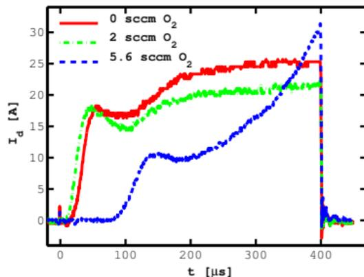
The current waveforms for an  $Ar/O_2$  discharge with a Ti target where the oxygen flow rate is varied – 600 V, 50 Hz and 0.6 Pa
