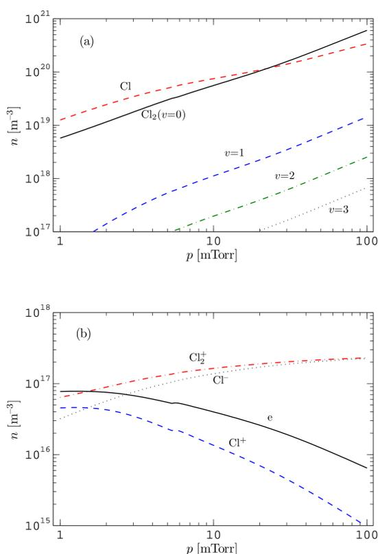
**Figure 2:** The density of (a) neutral chlorine species and (b) charged chlorine species versus discharge pressure at  $P_{\text{abs}} = 323$  W,  $Q = 100$  sccm,  $R = 18.5$  cm and  $L = 20$  cm.
