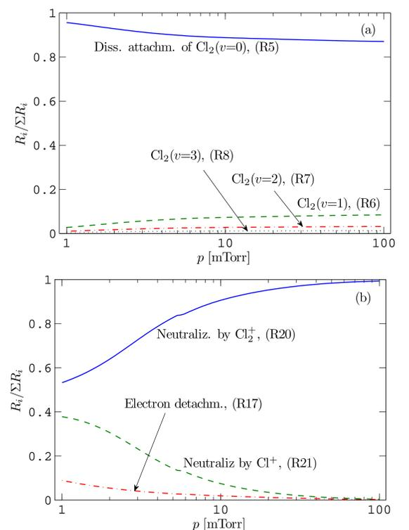
**Figure 5:** The relative reaction rates of (a) the creation and (b) the loss of the negatively charged chlorine ion  $\text{Cl}^-$  versus the discharge pressure at  $P_{\text{abs}} = 323$  W,  $Q = 100$  sccm,  $R = 18.5$  cm and  $L = 20$  cm.
