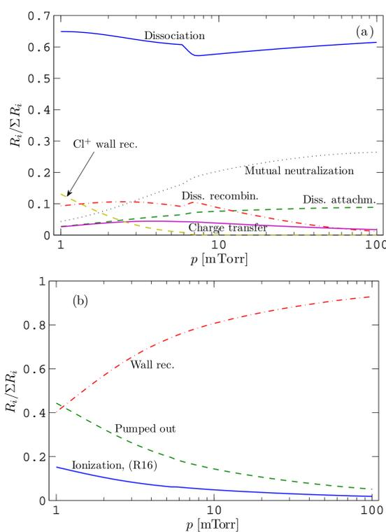
**Figure 4:** The relative reaction rates of (a) the creation and (b) the loss of the neutral chlorine atom Cl versus the discharge pressure at  $P_{\text{abs}} = 323$  W,  $Q = 100$  sccm,  $R = 18.5$  cm and  $L = 20$  cm.
