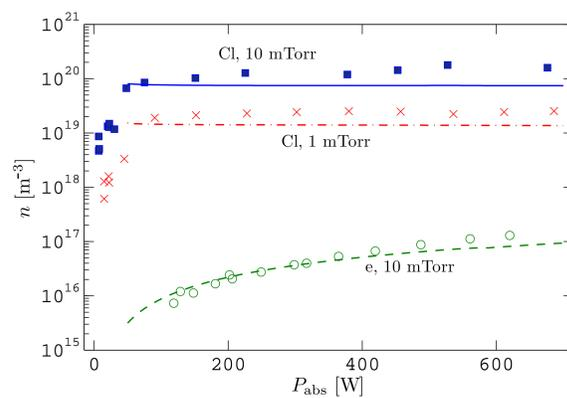
**Figure 3:** Model calculations of the atomic chlorine density at 10 and 1 mTorr (— and - - -) versus absorbed power compared to measurements (Malyshev and Donnelly, 2000, 2001) ( $\blacksquare$ ,  $\times$ ,  $\circ$ , respectively) at  $Q = 100$  sccm (20 sccm at 1 mTorr),  $R = 18.5$  cm and  $L = 20$  cm. A power coupling efficiency of 75 % was assumed for the measurements, i.e.  $P_{\text{abs}}/P_{\text{f}} = 0.75$ .
