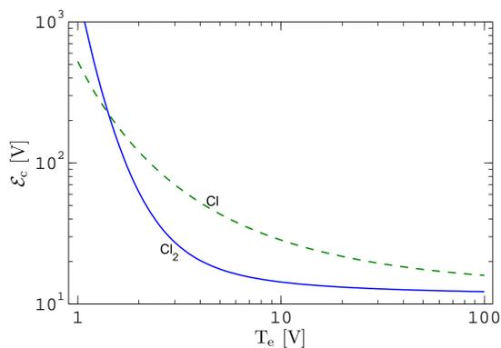
**Figure 1:** The collisional energy loss per electron-ion pair created  $\mathcal{E}_c$  as a function of the electron temperature  $T_e$  for the chlorine atom and the chlorine molecule.
