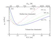
The power density is kept constant at  $P_{\rm abs}/V=79.6~{\rm kW/m^3}$  by varying the absorbed power  $P_{\rm abs}$  with R,L as indicated on the top axis.
