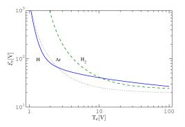
■ The collisional energy loss per electron-ion pair created for argon, hydrogen atoms and hydrogen molecules assuming Maxwellian EEDF
