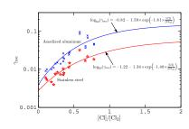
A fit to the measured data is for anodized aluminum
