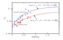
A fit to the measured data is for anodized aluminum
