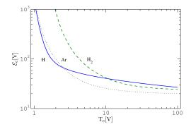
The collisional energy loss per electron-ion pair created for argon, hydrogen atoms and hydrogen molecules assuming Maxwellian EEDF
