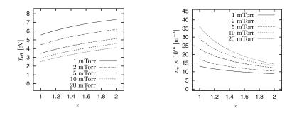
Particle balance gives the electron temperature
