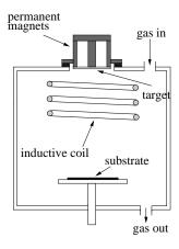
• In order to generate highly ionized discharge a radio-frequency discharge can be added in the region between the cathode and the anode
