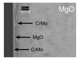
• A SEM image of  $\rm Cr_{0.63}Mo_{0.37}/MgO/Cr_{0.63}Mo_{0.37}$  MIM grown on MgO with 20 nm / 5 nm / 20 nm
