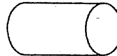
(b) Grind crystal to remove undulations and saw to remove portions not in resistivity range
