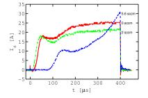
The current waveforms for an  ${\rm Ar/O_2}$  discharge with a Ti target where the oxygen flow rate is varied – 600 V, 50 Hz and 0.6 Pa
