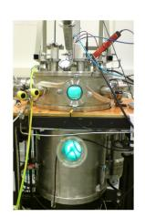
Planar Magnetron Sputtering Discharge
