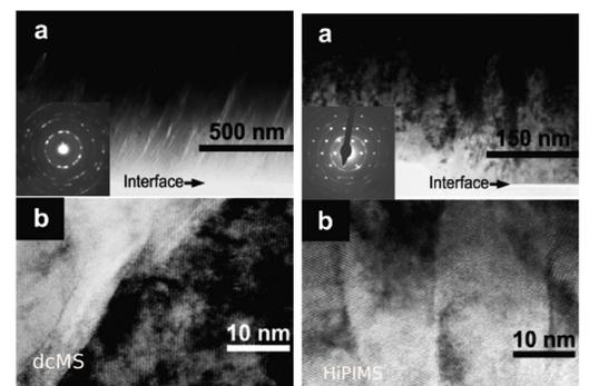
**Figure 4:** Ta thin films grown on Si substrates placed along a wall of a 2 cm deep and 1 cm wide trench by a dcMS and HiPIMS. (Left) dcMS grown films exhibit rough surface, pores between grains and inclined columnar structure, leaning toward the aperture and (Right) films grown by HiPIMS have smooth surface, and dense crystalline structure with grains perpendicular to the substrate. (From Alami et al. (2005)).
