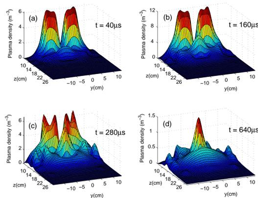
**Figure 2:** The spatial and temporal variation of the electron density in an argon discharge at 20 mTorr at (a) 40  $\mu$ s, (b) 160  $\mu$ s, (c) 280  $\mu$ s and, (d) 640  $\mu$ s, from initiating the 100  $\mu$ s long pulse. The target was made of titanium 150 mm in diameter. (After Bohlmark et al. (2005a))
