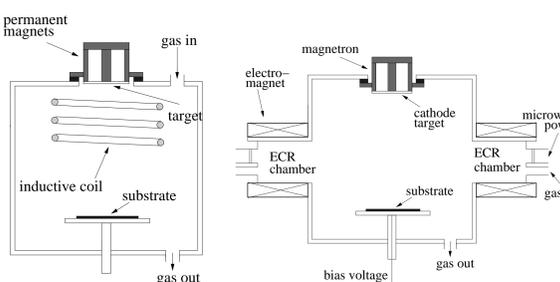
**Figure 1:** (Right) An ICP-MS where a radio-frequency-driven inductively coupled discharge is placed parallel to the cathode in between the cathode and the substrate. (Left) An ECR-MS apparatus, the two ECR discharge chambers are located at the opposite sites of the main processing chamber. (From Gudmundsson (2008)).
