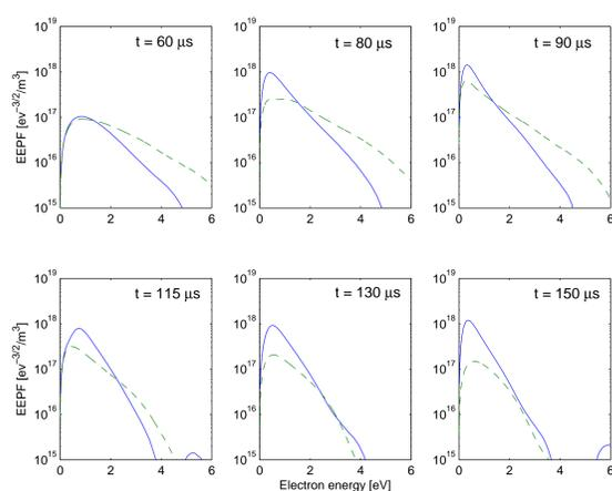
**Figure 3:** The electron energy probability function (EEDF) for various times from initiating the pulse for an argon discharge at 3 (green dotted line) and 20 (blue solid line) mTorr. The Langmuir probe is located under the race track 80 mm from the target surface. (From Gudmundsson et al. (2009)).
