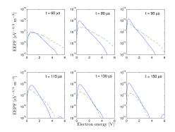
The electron energy probability function (EEPF) under the race-track 100 mm below the target for an argon discharge at 3 (dashed) and 20 (solid) mTorr with a copper target
