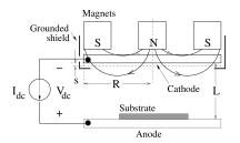
In magnetron sputtering, in order increase the lifetime of the electrons in the cathode target vicinity, magnets are placed behind the target surface  To account for the electrons that are not trapped we define an effective secondary electron emission coefficient
