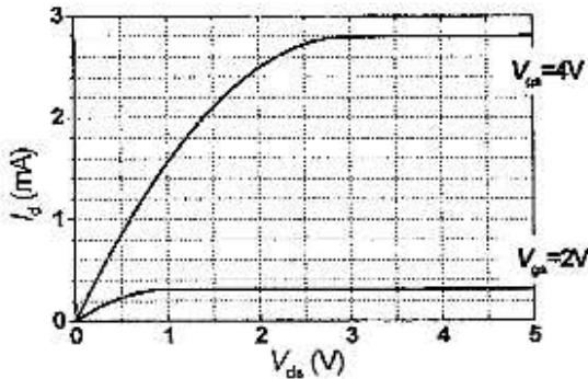
The following figure is the  $I - V$ -characteristics of an NMOSFET with  $d_{\text{ox}} = 10 \text{ nm}$ ,  $W = 10 \mu\text{m}$ ,  $L = 2 \mu\text{m}$ . (Do not consider velocity saturation)
